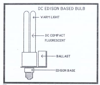
There are various shapes, sizes, styles and brands of AC and DC compact fluorescents both for diffused and spot lighting much the same as conventional incandescent bulbs. The only ones worth considering are those with the ballast built in and an Edison base (screw into a regular socket as shown above). All others end up requiring more technical labor to install and maintain than they are worth.
