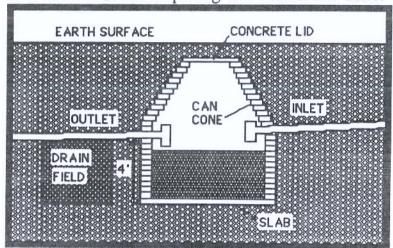
The lid will facilitate clean out which is a typical feature of all septic tanks although seldom ever needed in a "toilet only" septic tank. This lid can be buried under about 6" to 8" of soil.
