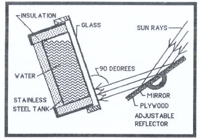
You want the reflectors (shiny metal or mirror on plywood) to be adjustable to reflect the sun so it hits the glass at a 90 degree or perpendicular angle. The sun reflects off of a surface at the same angle it comes in.
