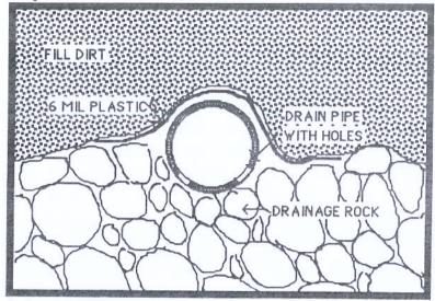
A layer of 6 mil plastic is usually placed over this to keep backfill dirt from seeping down into the gravel. This drain field is done exactly like that for a conventional septic tank if you wish to consult a local septic tank contractor. It is simply much shorter due to the fact that you are dealing with a significantly smaller volume of liquid.
