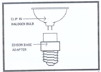
These adapt spot lights and many other types of lights to halogen use. Halogen lights however, are not as efficient as compact fluorescents. They are clearly a second choice on efficiency. Their selling point is that they provide more light with less wattage.
