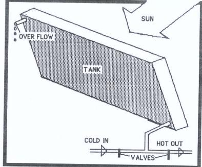
The valve arrangement shown can be located anywhere down in the dwelling. This tank is filled every morning and a few hours later (2 in the summer-4 in the winter) you have free hot water. Since the hot water is gravity fed to the taps the pressure is not very strong. This requires some custom easy flow fixtures or a mini
