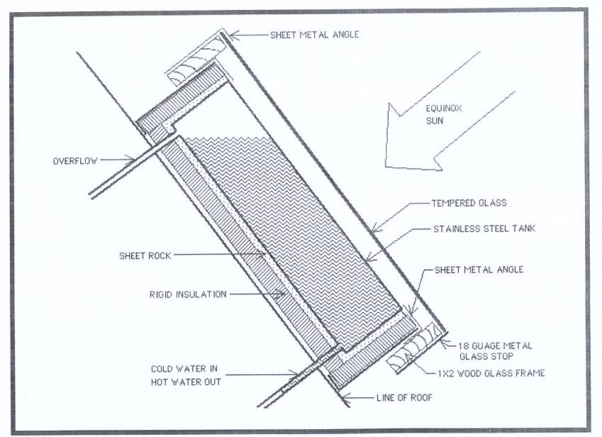
The above diagram shows actual construction detailing with a few more specifics than the
