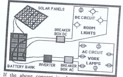
If the above concept is adopted, an occasional DC plug could still be added to the ROOM LIGHTING circuit to allow an occasional DC lamp. The "code required" AC plugs would still exist without interruption. The occasional DC plug on the room lighting circuit would simply be in addition to the DC room lighting.
